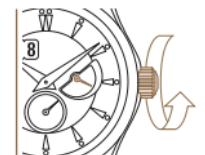
Rotate the crown clockwise until the power reserve indication hand has gotten at least to the middle of the scale.
