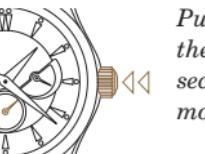
Push the crown back to the initial position. The second hand is back in motion.
